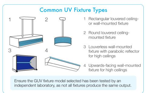
GUV can be used in a variety of ways within a healthcare setting, such as sterilizing equipment. To be used as a means of disinfecting air, GUV lights should be placed in appropriate fixtures and placed in the upper room (over the head of room occupants and not at eye level). These fixtures focus UV beams on the upper area of the room, preventing the minor irritation that can occur to eyes and skin when exposed to GUV.
